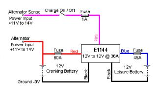
This Battery Charger has been designed using a building block system to obtain the power needed to suit your requirements
